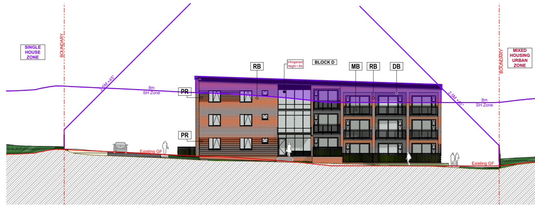
EL.08_ BLOCK D - NORTH ELEVATION
