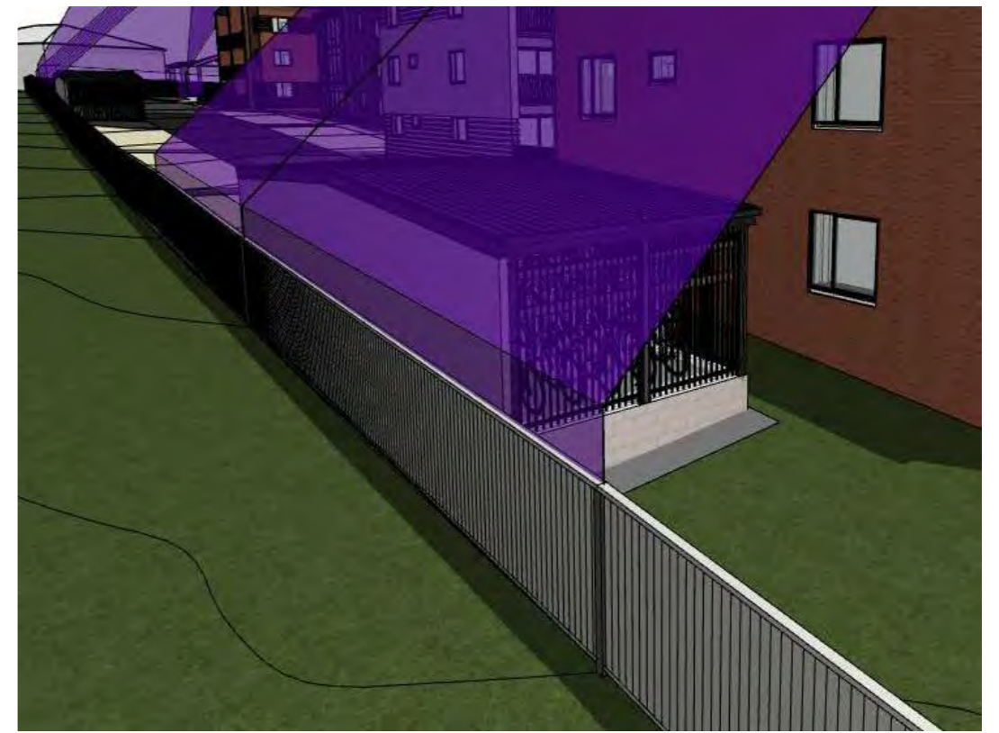
NORTHERN BIN AND BIKE STORAGE - NEXT TO BLOCK A - HIRB 2.5m + 45°
