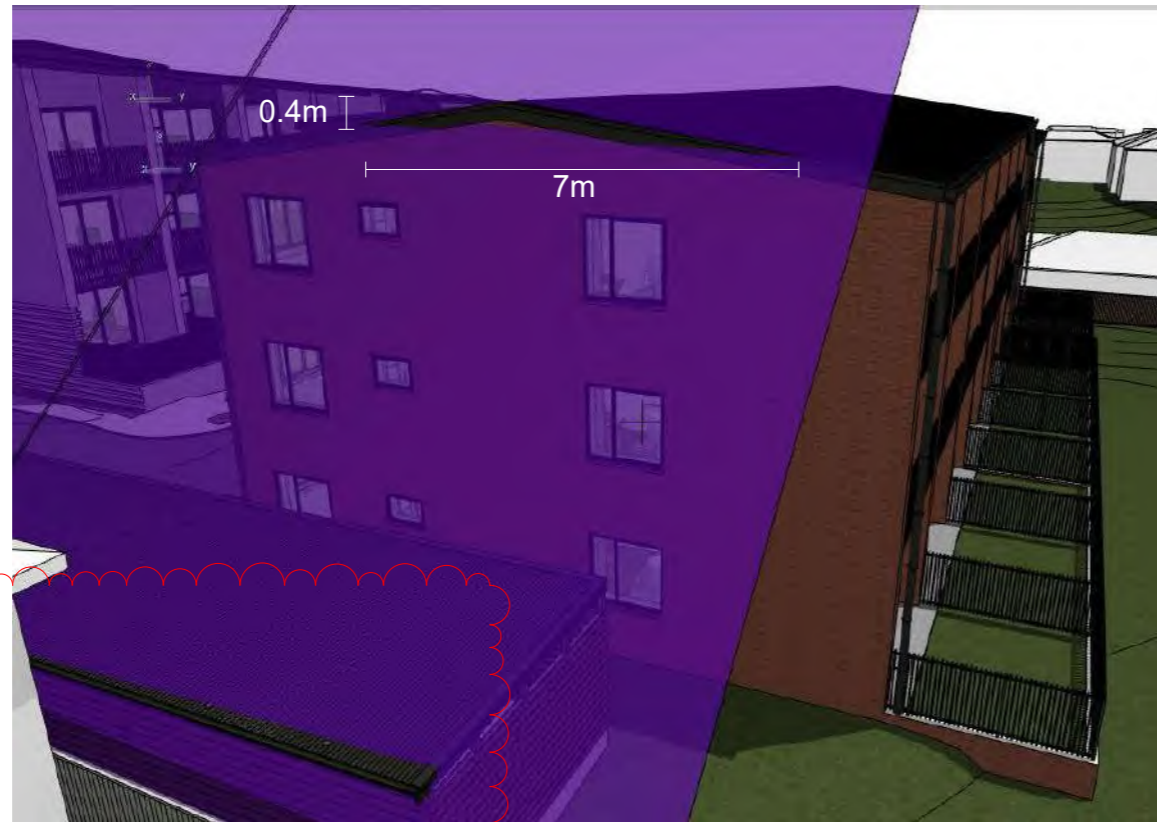
BLOCK A EASTERN FACADE - HIRB 2.5m + 45°
